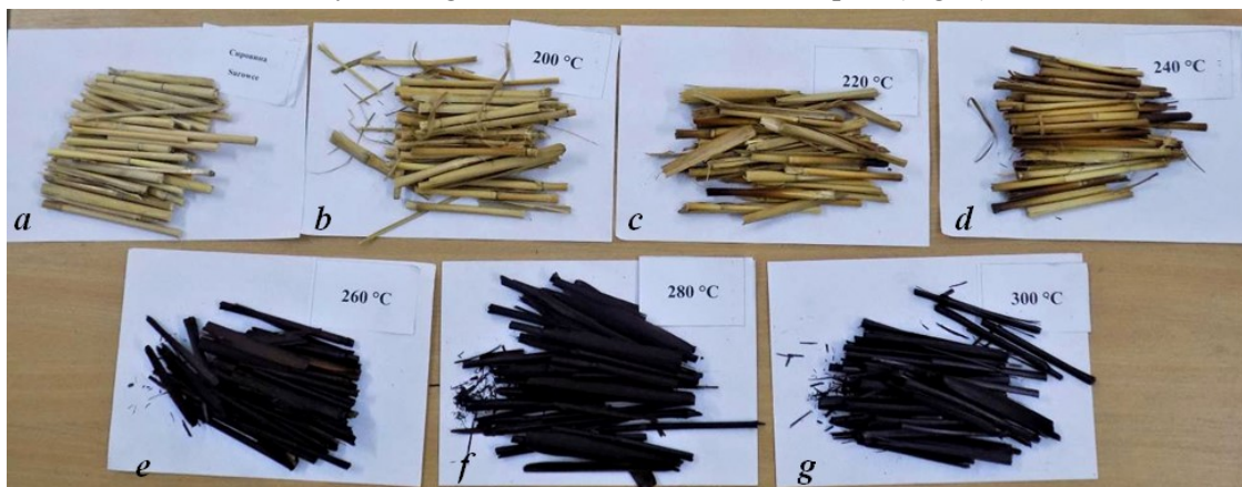
Fig. 3. General view of torrefied stems of Miscanthus Giganteus : a, b – 200 °C; c – 220 °C; d – 240 °C; e – 260 °C; f – 280 °C; g – 300 °C
